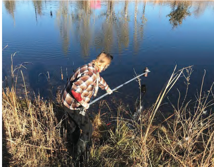
Figure 23-14. Grab sample being collected with a pool skimmer at Mead Pond.
